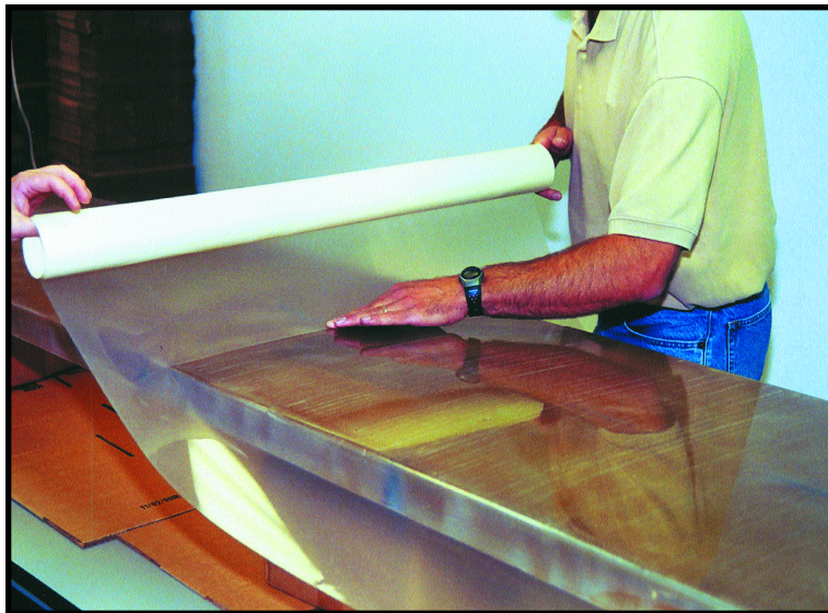
Operator applies a 5-mil ECTFE (Halar®) film treated on one side with 4 mils of PSA acrylic adhesive. The piece is a fiberglass baffle for an aqueous-media filter unit.
