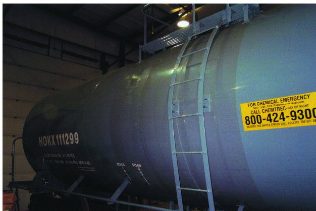
A 5-mil PVDF (Kynar®) film treated on two sides has been applied to this railcar using a 4-mil acrylic PSA adhesive. The film provides corrosion protection against splash and spillage during loading/unloading cars.
